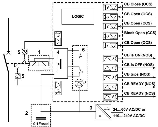
Figure 4: Block diagram of the control electronics
